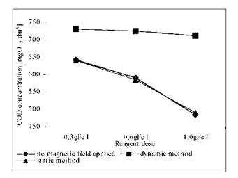
Fig. 9. Iron chloride impact on COD.
