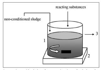
1. container with sludge; 2. magnetic stirrer; 3. sludge after conditioning.
