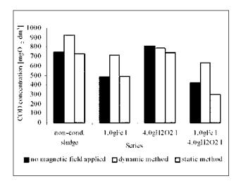
Fig. 5. Magnetic field impact on COD, at the highest doses of reacting substances.
