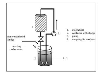
Fig. 2. Experimental stand in phase II (dynamic method).
